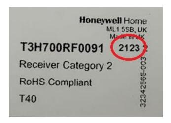
To access the date code on the wired T3, you will first need to remove the batteries from the front of the thermostat. Then, with a flat headed screwdriver, press down on the areas in the top corners of the battery compartments (as shown below). This will release the thermostat from the wall plate.
