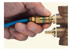
To remove the hose, pull the ring and remove. Done!
