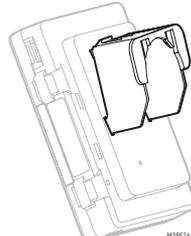
4. Slide the power supply into the holster
